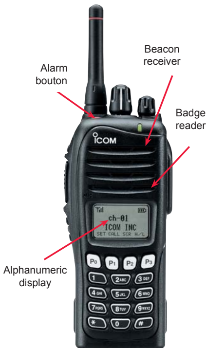
▲ Handheld radio short antenna (option) and keyboard. Existing without keyboard.
