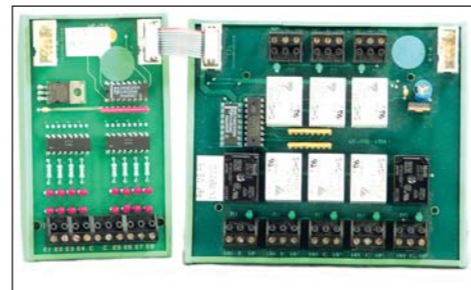
"Bus" assembly on another 8-input card and an 8-output relay card
