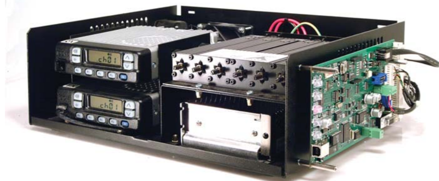
(Open) repeater equipped with IF-IT4 card (without covers).
