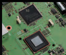
DSP + FPGA Unit (RF Deck)
