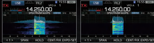
DPD OFF (Signal Received on the IC-7300) DPD ON (Signal Received on the IC-7300) No spurious emission observed
