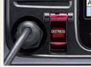
Distress button with a spring-loaded cover
