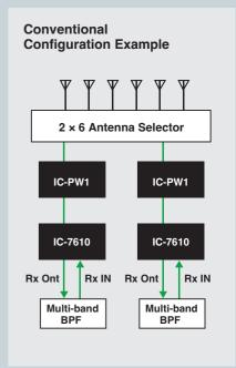
Multi-band Band-Pass Filters (BPFs) are used to prevent cross-band interference between your two radios during SO2R operation.
