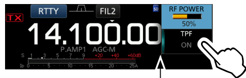
Lights while the TPF is ON
